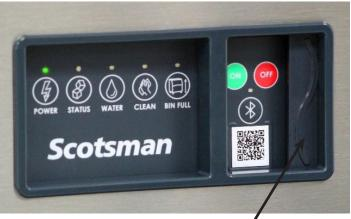
Open door to access On and Off switch buttons.
