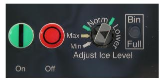
Rotate the adjustment post to the desired ice level.
